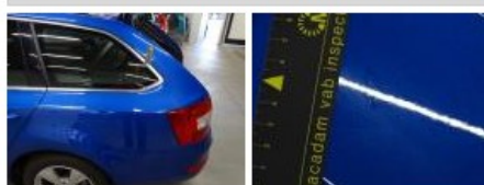
Door R R, Chemical polution, LI - Repair and paint (complete) 318,35
