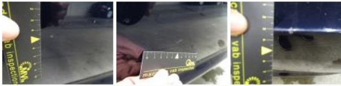
Wing F R, Stone chip(s), Acceptable 0,00
