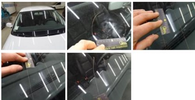
Bonnet, Chemical polution, LI - Repair and paint (complete) 0,00
