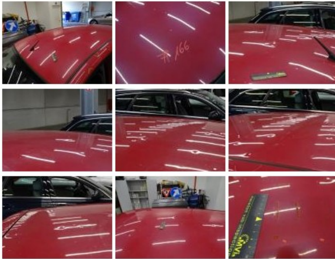
Roof pillar L, Hail damage, PDR - Hail 450,00
