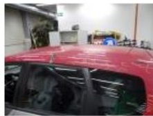
Roof pillar L, Hail damage, PDR - Hail 450,00
