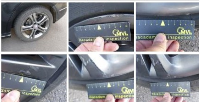
Door R R, Bump(s) and scratch(es), Acceptable
