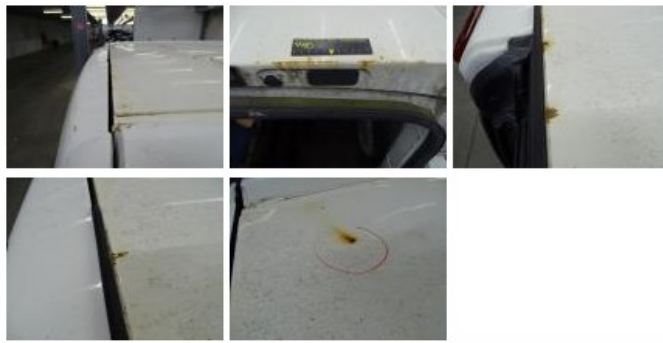
Wing R R, Bump(s) and scratch(es), LI - Repair and paint (complete) 231,15
