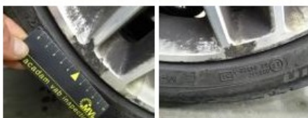
Wing R R, Scratch(es), LI - Repair and paint (complete) 308,20
