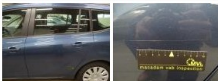
Door F R, Bump(s) and scratch(es), LI - Repair and paint (complete)
