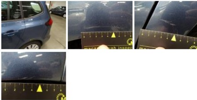
Wheel cover R L, Scratch(es), E - Replace
