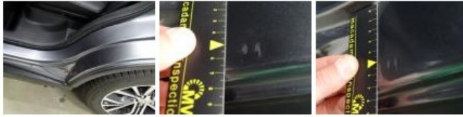
Door frame R L, Bump(s) and scratch(es), It - Spot repair
