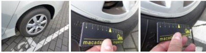
Alloy rim R L, Scratch(es), LI - Repair and paint (complete) 95,00
