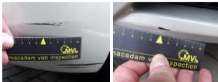
Outer door handle F L, Damaged, Le - Replace and paint 0,00
