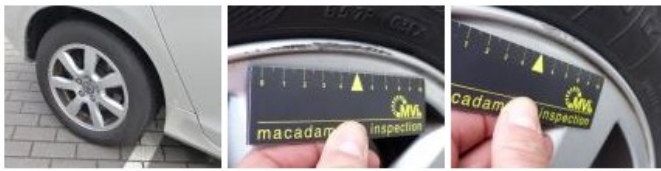
Alloy rim R L, Scratch(es), LI - Repair and paint (complete) 95,00
