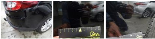
Rearlight R , Crack, E - Replace 114,00
