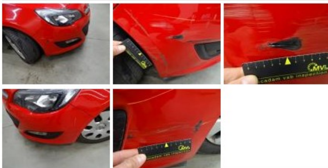
Door F L, Bump(s) and scratch(es), LI - Repair and paint (complete) 318,35
