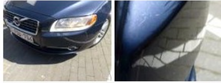
Grill frame, Broken, E - Replace
