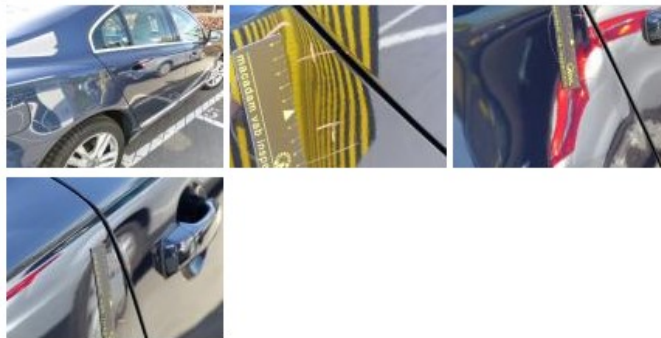
Sill outer R, Scratch(es), It - Spot repair
