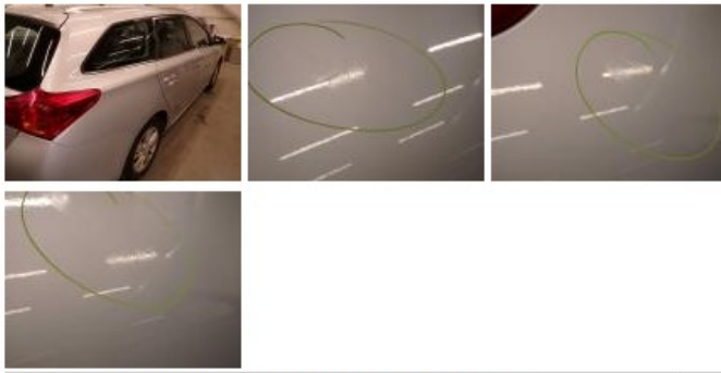
Door frame F R, Bump(s) and scratch(es), It - Spot repair 0,00
