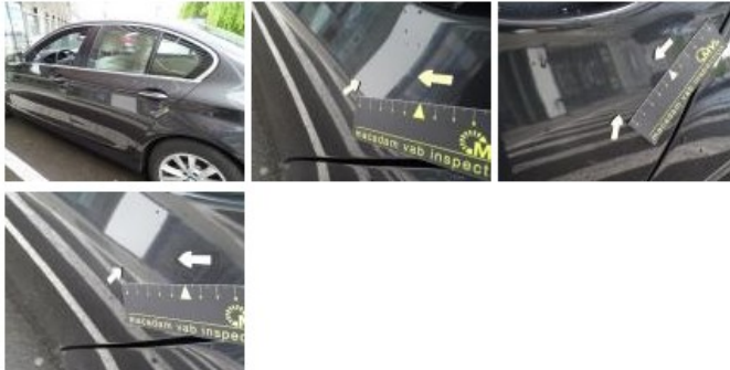
Door R R, Bump(s) and scratch(es), LI - Repair and paint (complete) 430,02
