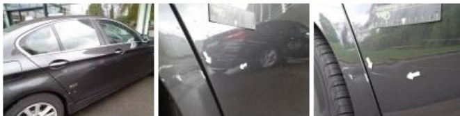
Sill trim R, Scratch(es), LI - Repair and paint (partial) 0,00
