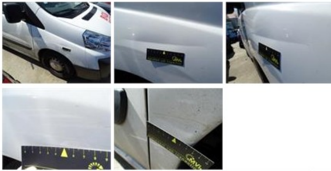
Wing F L, Bump(s) and scratch(es), LI - Repair and paint (complete) 165,13
