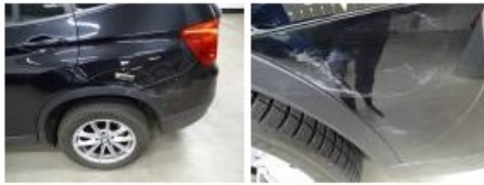
Door R R, Scratch(es), LI - Repair and paint (complete) 382,02
