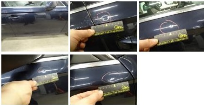
Door R R, Bump(s) and scratch(es), LI - Repair and paint (complete) 382,02
