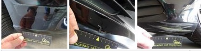
Wing R L, Scratch(es), LI - Repair and paint (complete) 0,00
