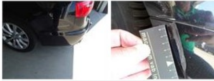
Front bumper, Scratch(es), LI - Repair and paint (complete) 0,00
