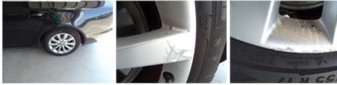
Alloy rim R L, Scratch(es), LI - Repair and paint (complete) 0,00
