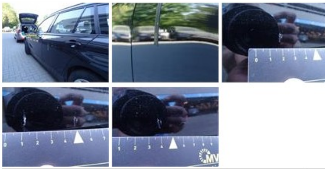
Door F L, Scratch(es), LI - Repair and paint (complete) 318,35
