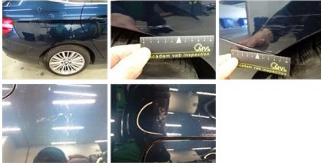
Roof pillar R, Chemical polution, LI - Repair and paint (complete) 220,18
