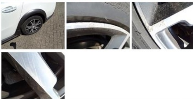
Alloy rim F L polished, Damaged, E - Replace 235,20
