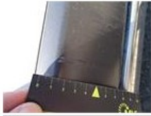
Door R R, Bump(s), PDR - Knock out without painting 63,00
