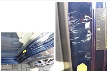
Wing F R, Bump(s), LI - Repair and paint (complete)
