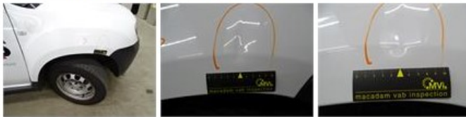
Sill outer R, Damaged, Le - Replace and paint 298,00
