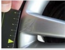
Alloy rim F R, Damaged, E - Replace
