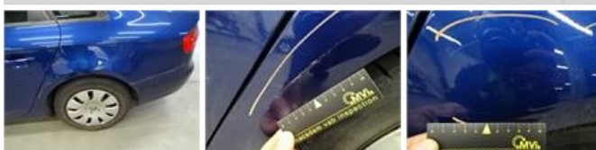
Protection plate M, Tear, E - Replace 74,00
