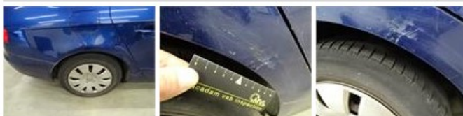
Door R R, Scratch(es), LI - Repair and paint (complete) 318,35
