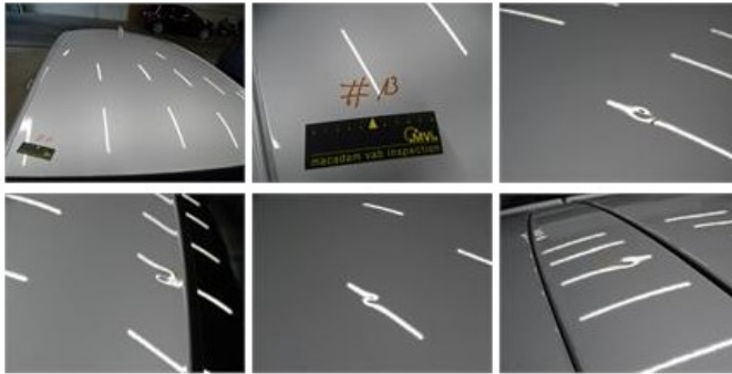
Roof, Hail damage, PDR - Hail 325,00
