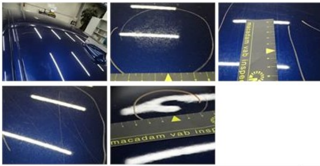
Wing F R, Bump(s) and scratch(es), Le - Replace and paint 530,02
