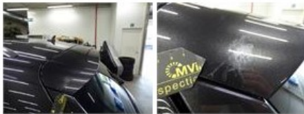
Wing R L, Chemical polution, LI - Repair and paint (complete) 369,84
