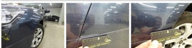
Door F R, Scratch(es), LI - Repair and paint (complete) 318,35
