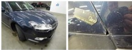
Door F L, Scratch(es), LI - Repair and paint (complete) 318,35
