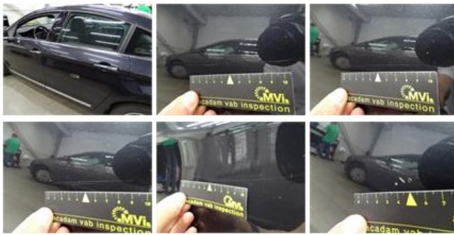
Wing F R, Bump(s) and scratch(es), LI - Repair and paint (complete) 220,18
