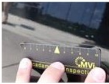
Door R L, Bump(s) and scratch(es), LI - Repair and paint (complete)
