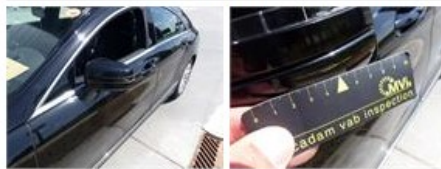
Door R R, Bump(s) and scratch(es), LI - Repair and paint (complete)
