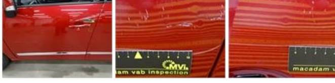
Door F L, Bump(s) and scratch(es), LI - Repair and paint (complete) 318,35
