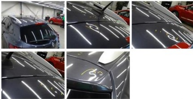
Wing R L, Hail damage, PDR - Hail 100,00
