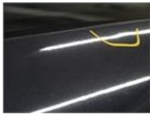
Door R L, Hail damage, PDR - Hail 75,00
