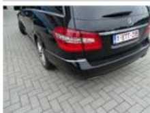
Bumper R, Scratch(es), LI - Repair and paint (complete) 254,16
