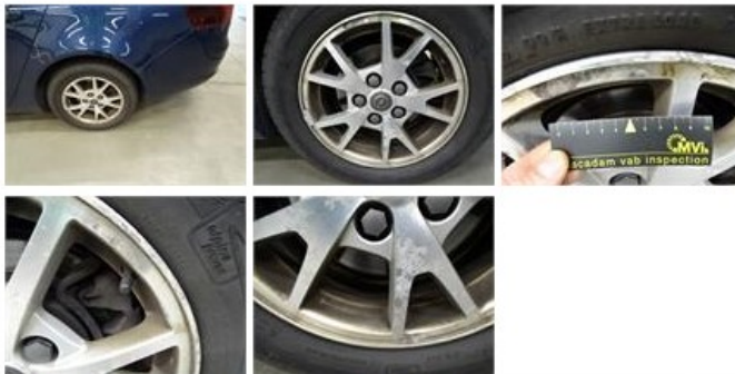
Alloy rim F R, Rust, LI - Repair and paint (complete) 95,00
