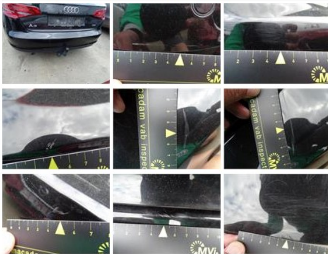
Wing R R, Bump(s) and scratch(es), LI - Repair and paint (complete) 308,20
