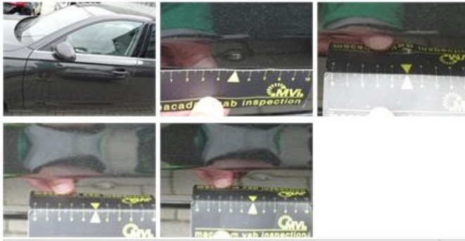
Wing R R, Bump(s) and scratch(es), LI - Repair and paint (complete) 369,84
