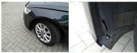
Door F L, Bump(s) and scratch(es), LI - Repair and paint (complete) 382,02
