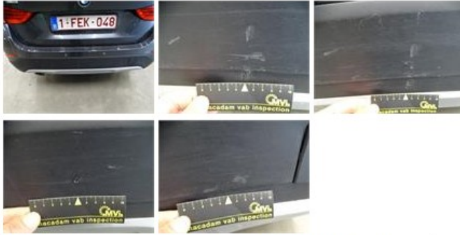
Door R L, Bump(s) and scratch(es), LI - Repair and paint (complete) 318,35
