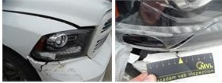
Headlight R, Damaged, E - Replace
