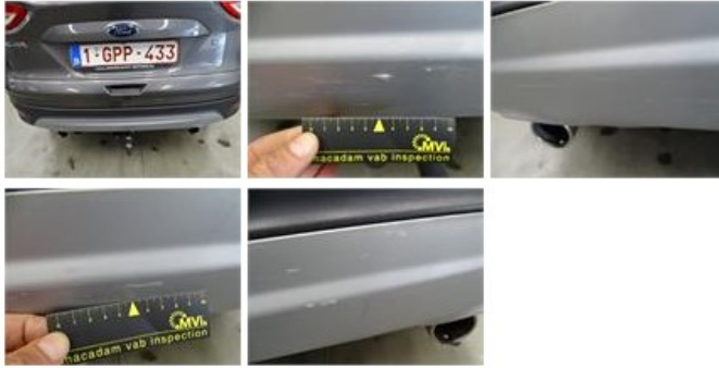
Tailgate, Scratch(es), LI - Repair and paint (complete) 362,02
