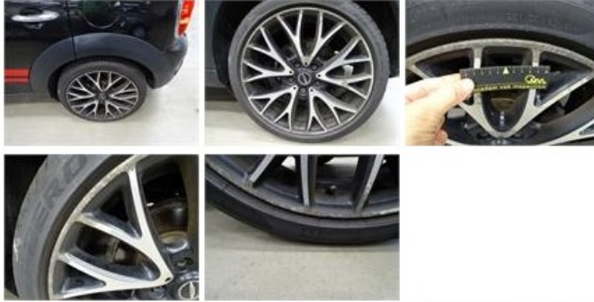
Alloy rim F L polished, Scratch(es), LI - Repair and paint (complete) 95,00
