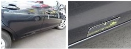
Door frame R L, Scratch(es), It - Spot repair
