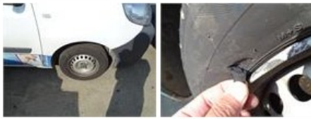
Steel rim R L, Damaged, E - Replace
