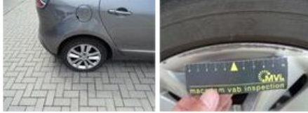
Alloy rim R R, Scratch(es), LI - Repair and paint (complete) 95,00
