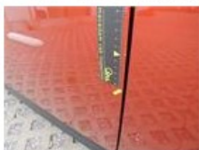
Roof, Stone chip(s), Acceptable 0,00
