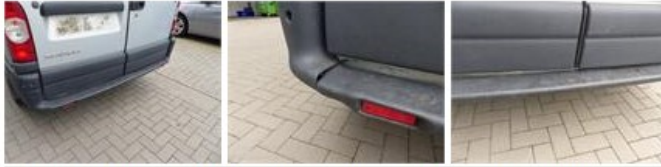
Sill outer R, Bump(s) and scratch(es), LI - Repair and paint (complete)
