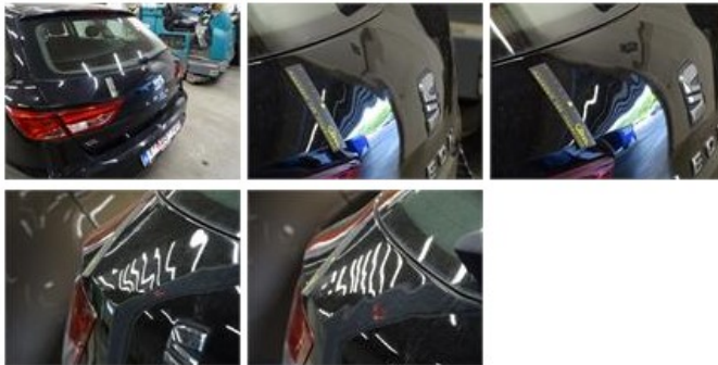
Door R R, Scratch(es), LI - Repair and paint (complete) 0,00
