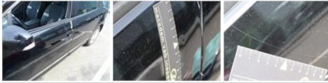
Door frame R L, Bump(s) and scratch(es), It - Spot repair 115,56
