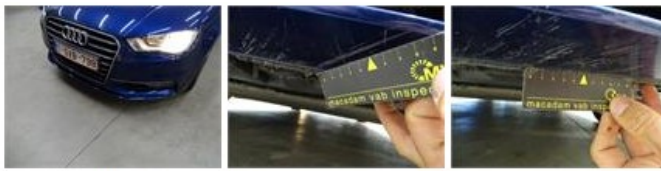
Bumper grille, Broken, E - Replace 32,40
